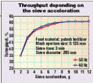
**FIGURE 4.** Even at identical amplitude settings, the “g” force will vary slightly, as a function of the frequency of the mains supply and should always be considered when comparing results between countries with different frequencies. A good sieve shaker will allow precise setting of the amplitude and g forces
