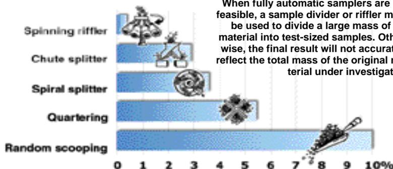
**FIGURE 2.** A number of sampling techniques are available — each achieving a particular degree of accuracy, as indicated above by their deviations from the mean size
