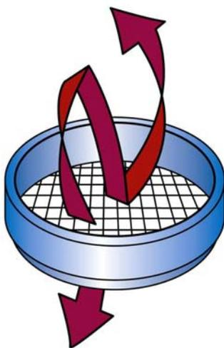
*Fig.: The electromagnetic drive of the AS 200 and AS 300 "control" ensures a 3-dimensional throwing movement that allows the sample to wander uniformly across the whole surface of the sieve.*
