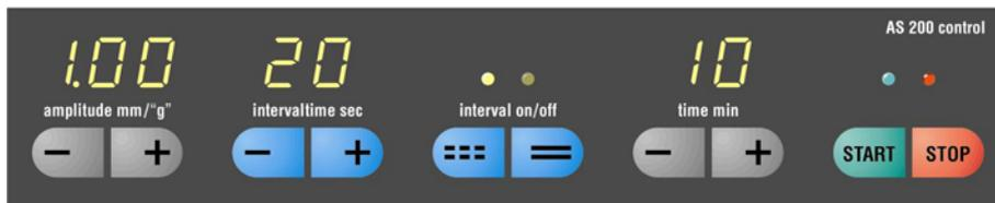
Fig.: Digital setting of the oscillation amplitude on the AS 200 "control" from Retsch
