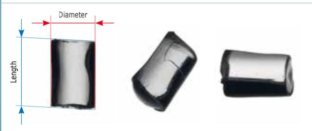
Thanks to the new, brighter light source and the high resolution cameras transparent particles can be captured with excellent contrast, enabling accurate and precise detection. The example above shows the length and the diameter analysis of transparent pellets.
